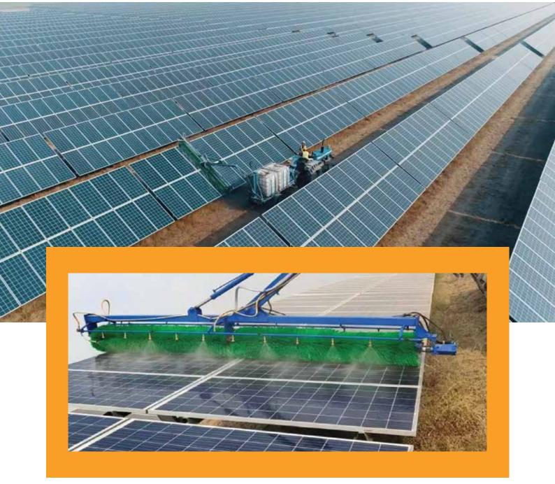
Inhouse module cleaning system developed by Azure Power.
